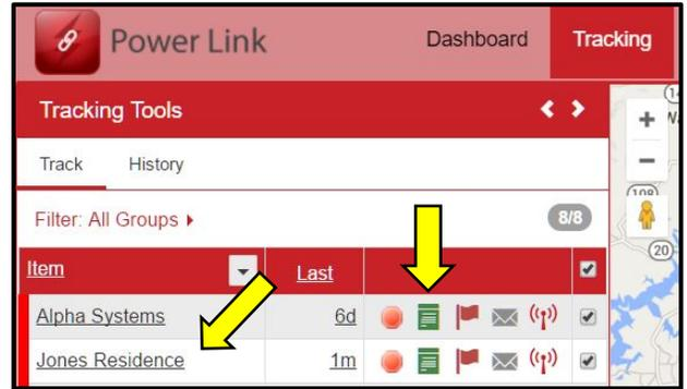
**Test Input Connections:** Once the monitor is communicating with the Power Link user interface, you will be able to see the events sent from the monitor. It is a good idea to test the input connections before leaving to make sure that the inputs are wired correctly and functioning properly. Test each input and verify that the events are being received.
