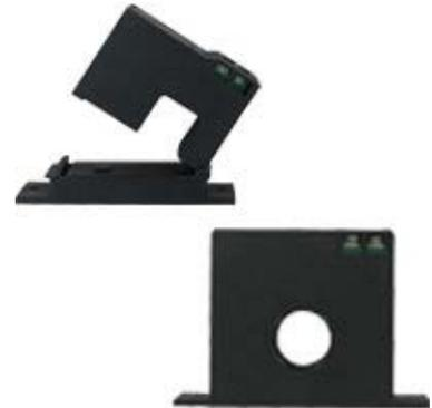
The generator current sensing switch can be installed on either side of the generator main line circuit breaker. The current switch can be installed on any Leg/Line as it will sense the presence of current whenever the generator is under load. The current switch has a dry contact relay for use with the input leads on the monitor.
